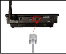
**Step 2**Connect the ES Receiver serial cable to the serial port on the back of the ISTATION and then tighten the screws.
