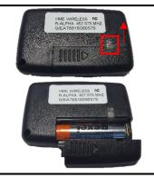
On the back, push the clear lock up to unlock the battery cover. Slide the battery cover off. Once opened, insert battery. Slide the cover back on and push the clear lock down to secure the battery cover in place.
