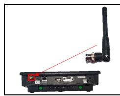
**Step 1**Connect the antenna to the transmitter.
