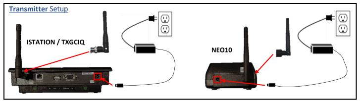
Step 1 Connect the antenna to the transmitter. Twist to lock in place.
